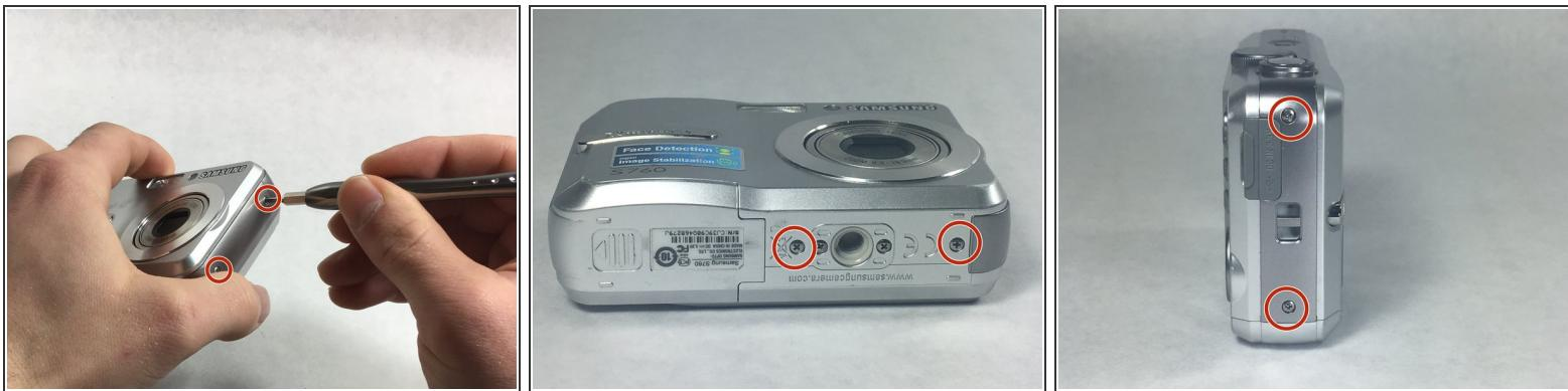
**i** All screws in this camera are removed using the Phillip Screwdriver #000 bit. Also, all dimensions included refer to screw *lengths*.
