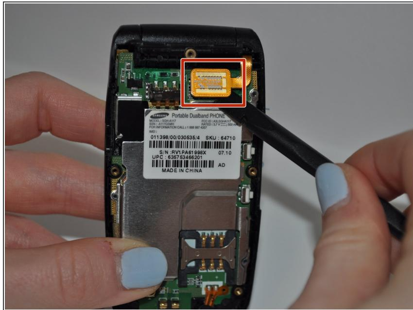
**i** Use the metal prying tool to gently flick up the rectangular connector. (Because this device is on the smaller side, the rectangular connector may only need a simple flick with the prying tool)
