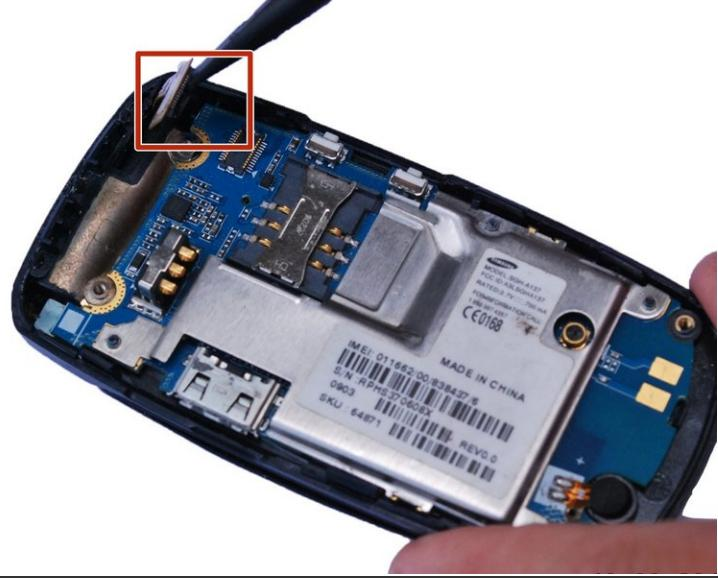
*(i)* Smaller press-fit connectors may require a simple flick with a plastic opening tool or spudger.
