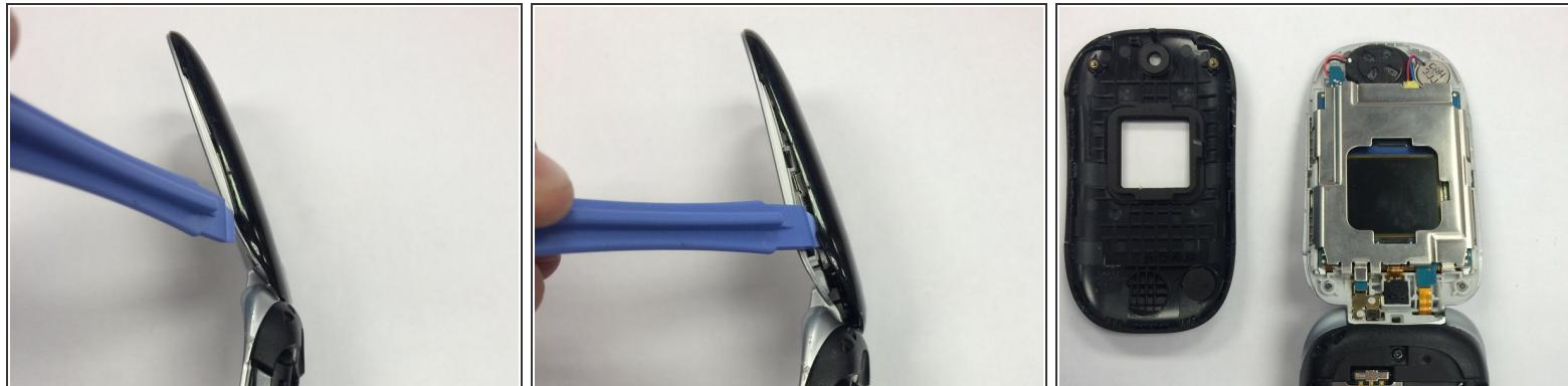
! Failure to utilize the specified tool may cause damage to the device.
