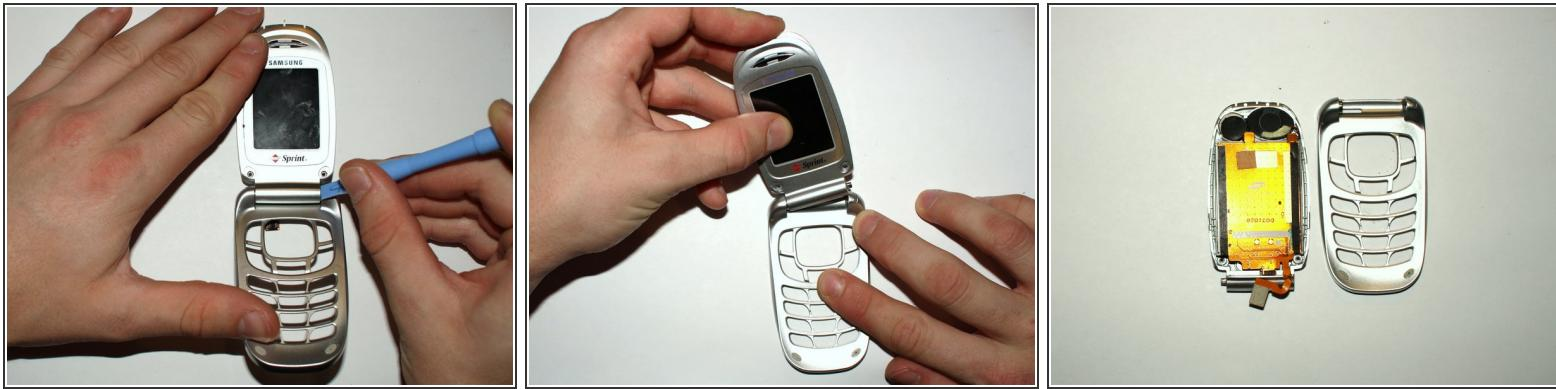
**⚠ Be Extremely Careful** in this next step as if you pry the hinge off too fast you may rip the connector between the logic board and screen.
