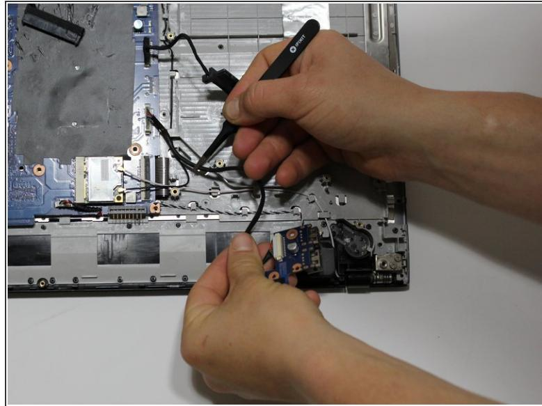
**⚠** Using the tweezers, gently pry up the chip and ports, and unthread the wire from its holders, without crimping the wires.
