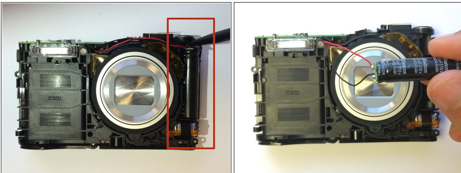
**⚠ Caution:** Touching the capacitor wires may cause serious injury. Use a [capacitor discharge probe](#) to safely rid the capacitors of dangerous charges.
