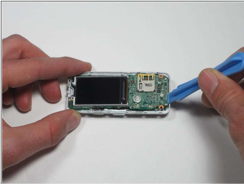
**⚠ CAUTION:** Do not scrape the spludger along the top of the motherboard or you may damage the circuitry.
