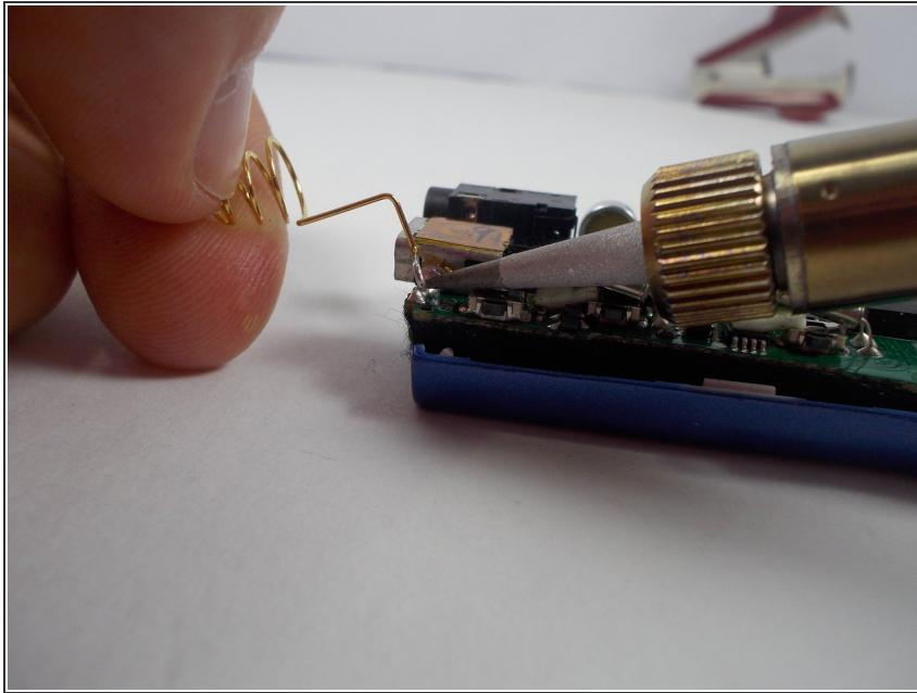
ⓘ There may be some solder in the way of the spring contacts' metal contacts. If this occurs simply melt the solder to create room for the contacts.
