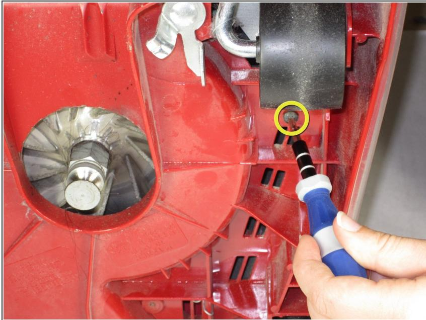
**⚠** Be sure to unplug the vacuum before disassembling it to prevent electric shock.
