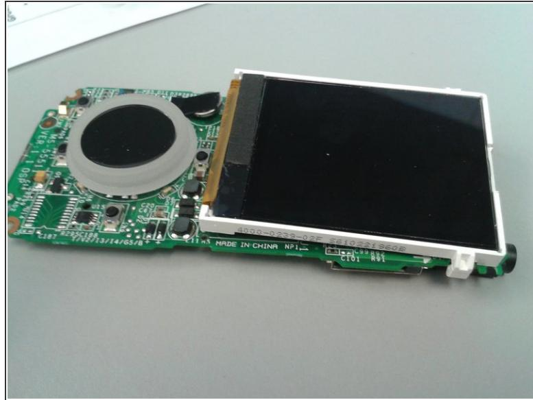
**⚠** This is as far as you can go without specialized board rework equipment. Trying to forcibly remove the screen will destroy it, but you can gently move it aside for cleaning or access to other board components.
