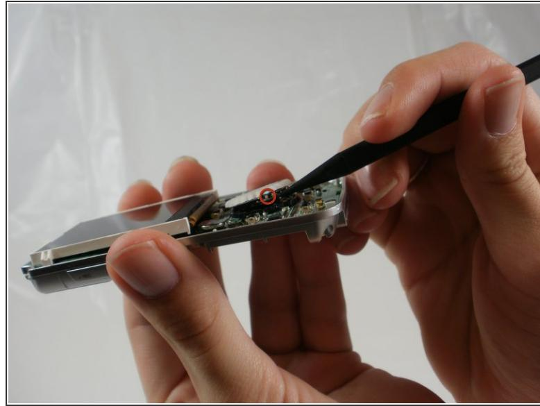
*(i)* There are 4 small metal hooks under the white scrolling mechanism.
