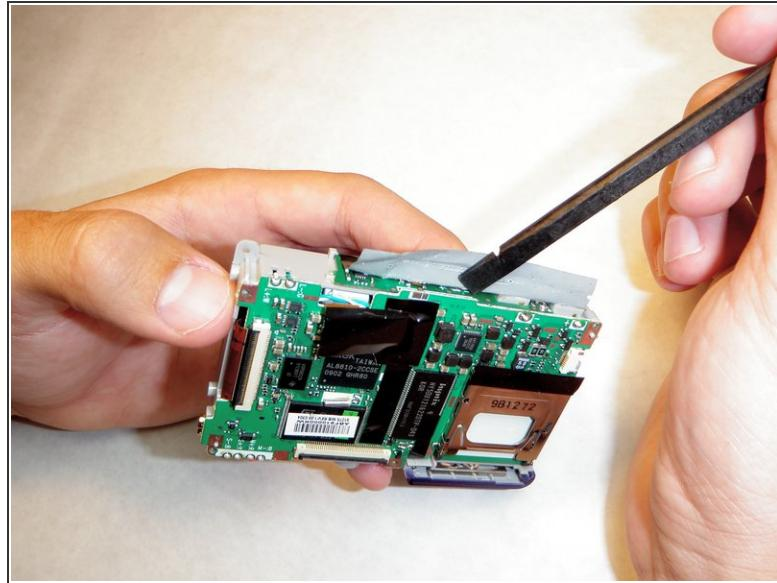
**⚠** Do not touch ANY part of the logic board previously covered by the black film until the capacitor has been completely discharged. This camera has a 330V, 100  $\mu$ F capacitor which can cause painful electric shock.
