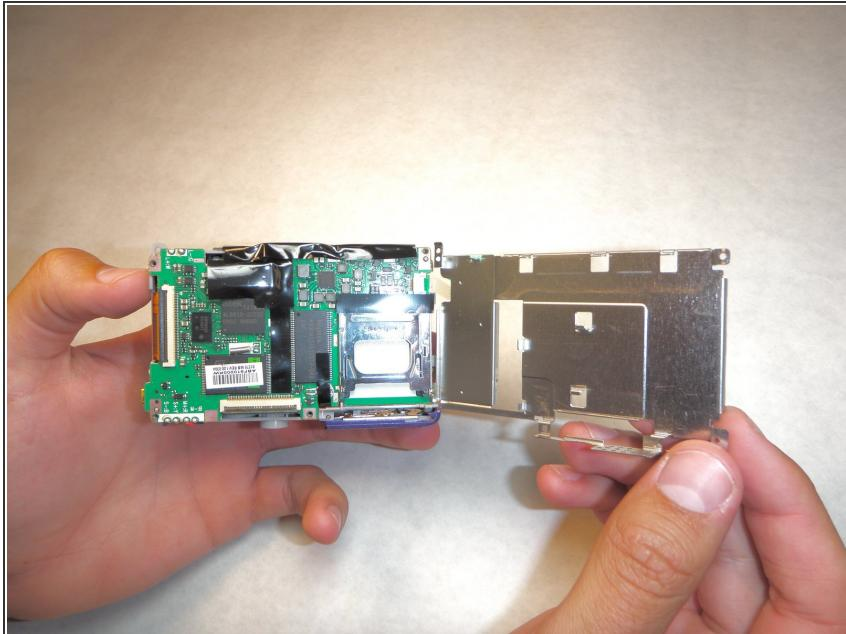
⚠ Be careful when rotating the plate in the next step to prevent the ribbon cable in the top right from ripping.
