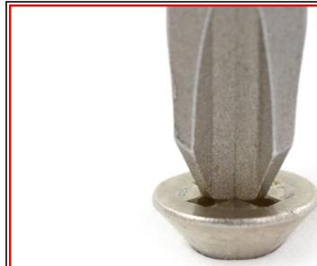
ⓘ A correctly sized driver should “fill up” the screw head, utilizing both the full depth and width of the socket.
