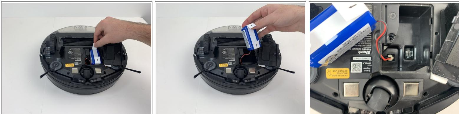
ⓘ Be careful when removing the battery, as it will still be connected to a wire.
