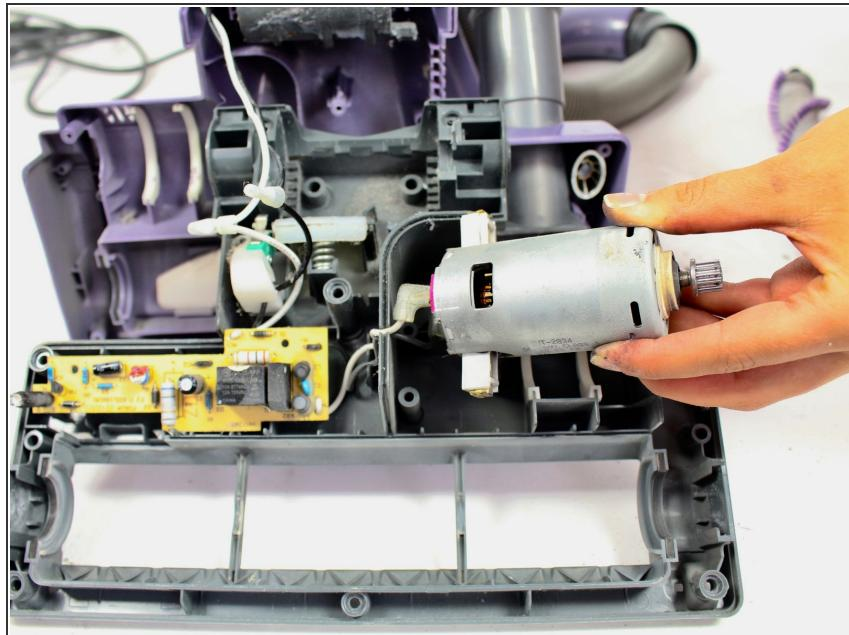
⚠ The wires are attached to the motor, so take out the motor slowly to ensure that they do not break.
