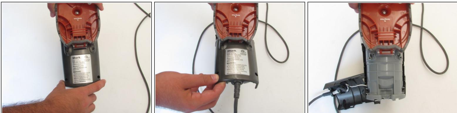
! Removing the gray panel reveals the wiring to the fan and motor, be careful not to pull too hard on the wires to break or disrupt them.
