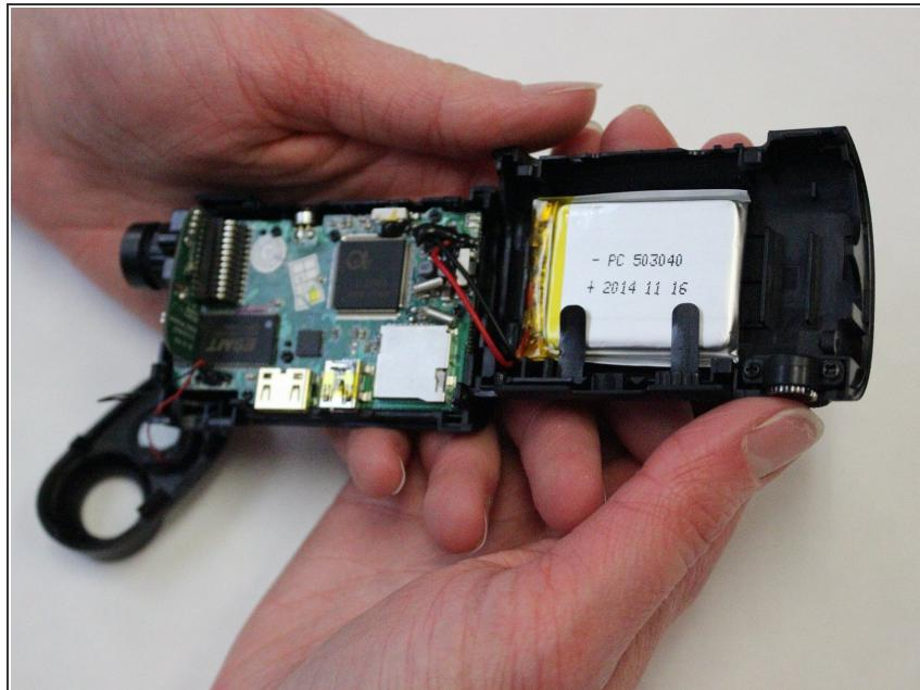
**⚠** Be gentle with the device since there are wires attached to the front plate and two halves.
