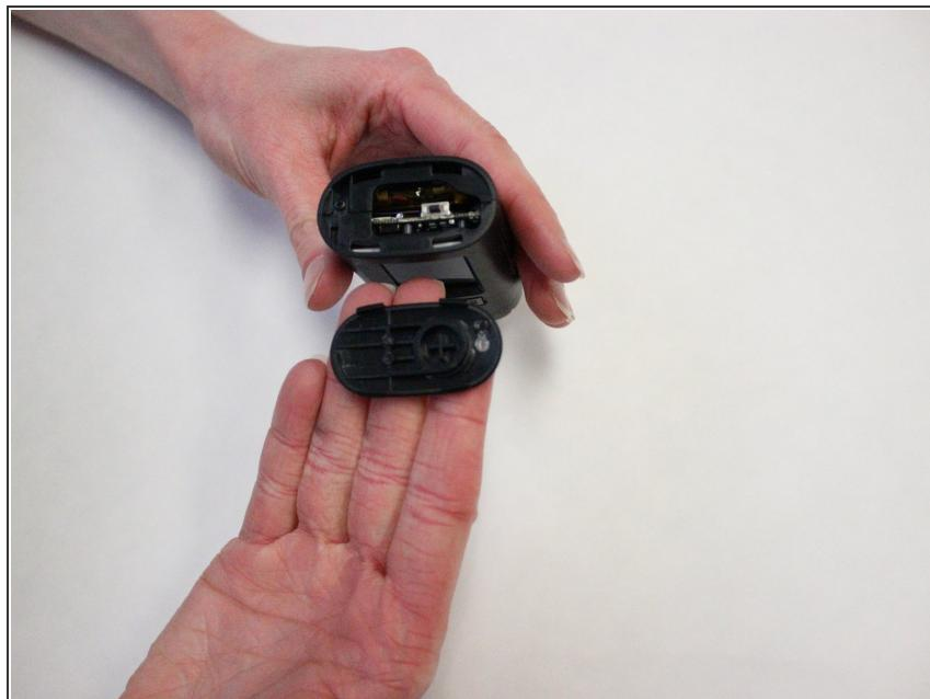
*(i)* To replace the on/off button, you must replace the entire back panel. The on/off button cannot be removed from the panel.
