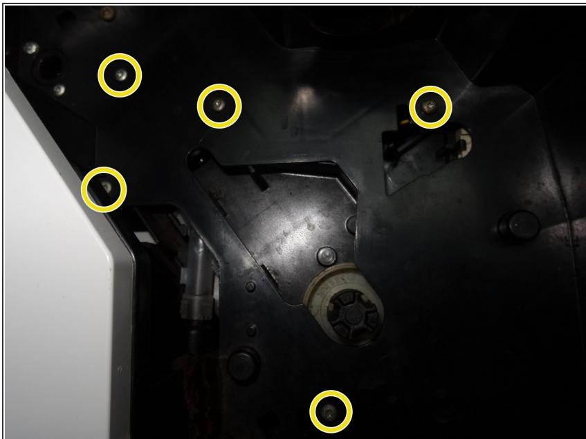
ⓘ The drainage valve is directly plugged to the gear drive. The drive is fixed with five Torx T10 screws on the center panel behind the brew group.
