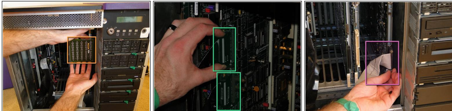
**⚠** Whenever working inside the machine, prevent ESD (electrostatic discharge)! Wear a conductive wrist strap and avoid insulating clothes such as wool, nylon, or synthetic material. Only place boards on a non-conductive bag or anti-static working mat.
