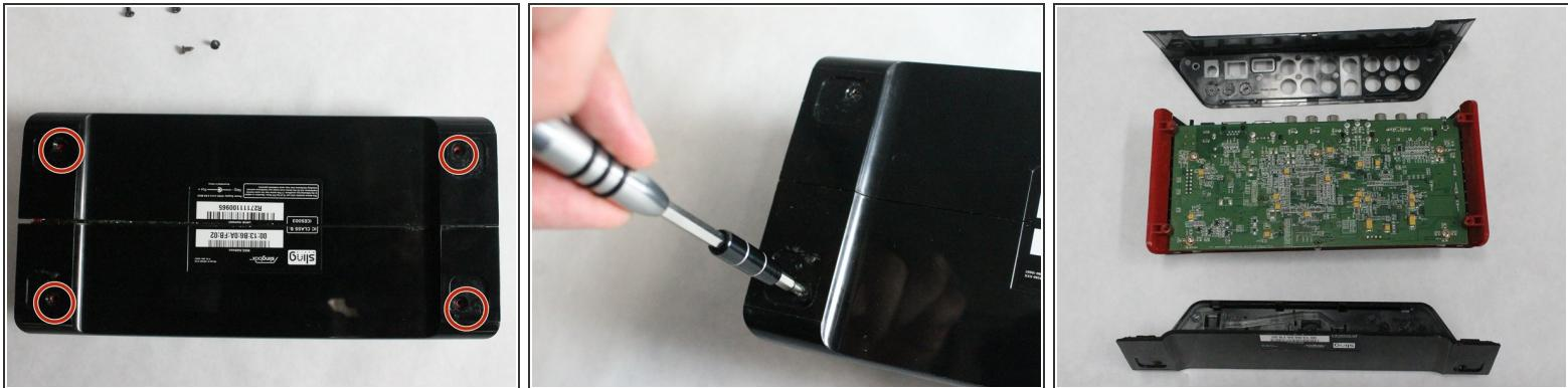
*(i)* The Slingbox has four black 5mm screws, one on each corner of the case.
