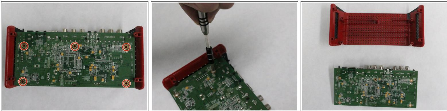
*(i)* The motherboard has five silver 5.5mm screws connecting it to the base of the Slingbox.
