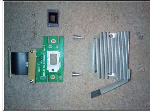
**⚠** Before removing the DMD heatsink, clean any dust from the area to prevent dust getting into the optical system.
