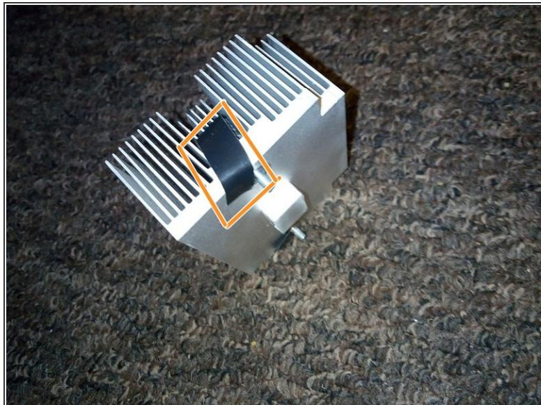
⚠ A poor thermal contact between the DMD chip and the heatsink could lead to premature failure of the chip. This projector uses thermal tape between the chip and the heatsink to ensure a good thermal contact.
