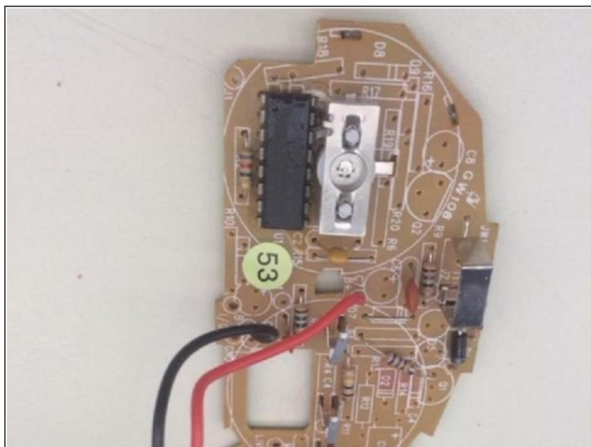
⚠ The metal cap is removed to reveal a, MC145017, driver chip and americium sensor. Do not remove americium from the sensor!
