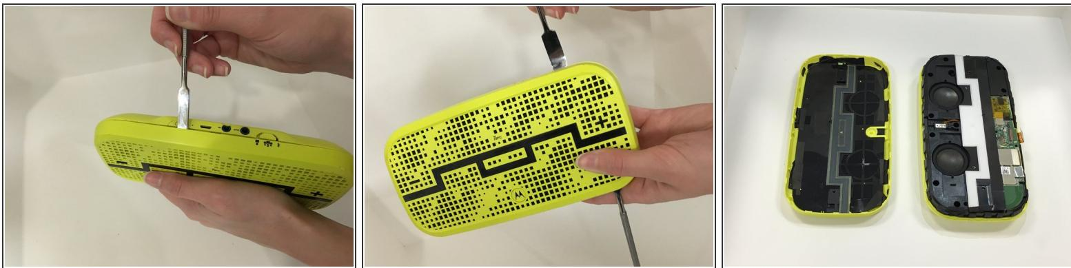
**⚠** When working with electronics, it's important to choose a tool that's ESD-safe to avoid accidental damage to the device. The regular black nylon spudger or a plastic opening tool should be used whenever possible.
