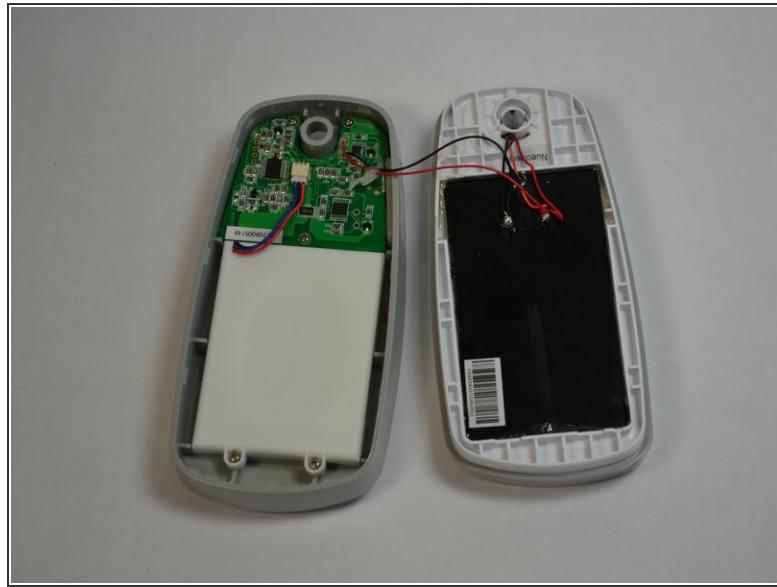
**⚠** Do not fully pull apart the back panel from the device. Doing so can rip the two red and blue wires attached to the panel.
