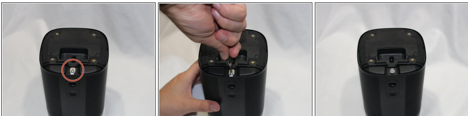
*(i)* The protective cover clip is very thin and deforms easily.
