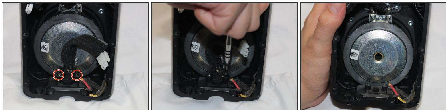
*(i)* The woofer is highly magnetic, making removal of the metal screws sometimes difficult.
