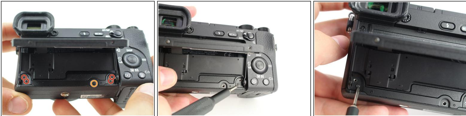
**i** To access the LCD assembly we need to remove the screws attaching its hinge to the camera body.
