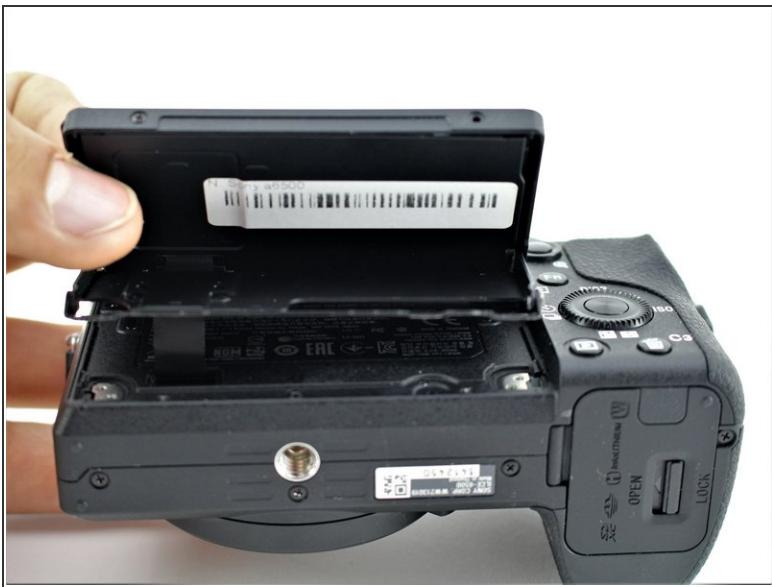
*(i)* To access the back of the camera remove the screws attaching the LCD screen hinge to the camera body.
