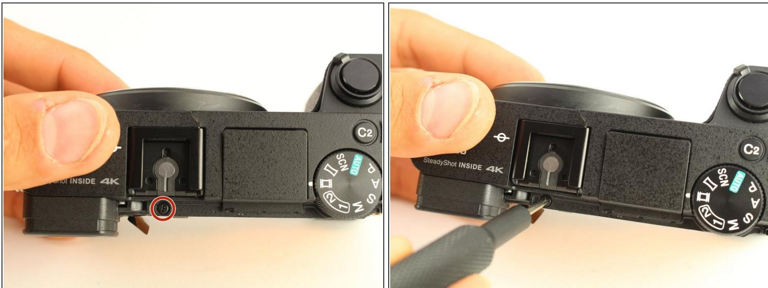
*(i)* The last screws holding the top on can be accessed once the back of the camera is removed.
