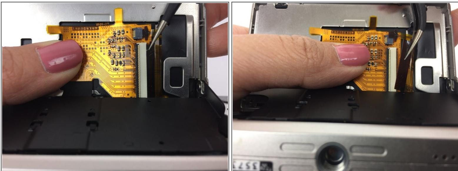
**⚠** Remove the larger ribbon cable. This may require extra force that could damage the ribbon cable.
