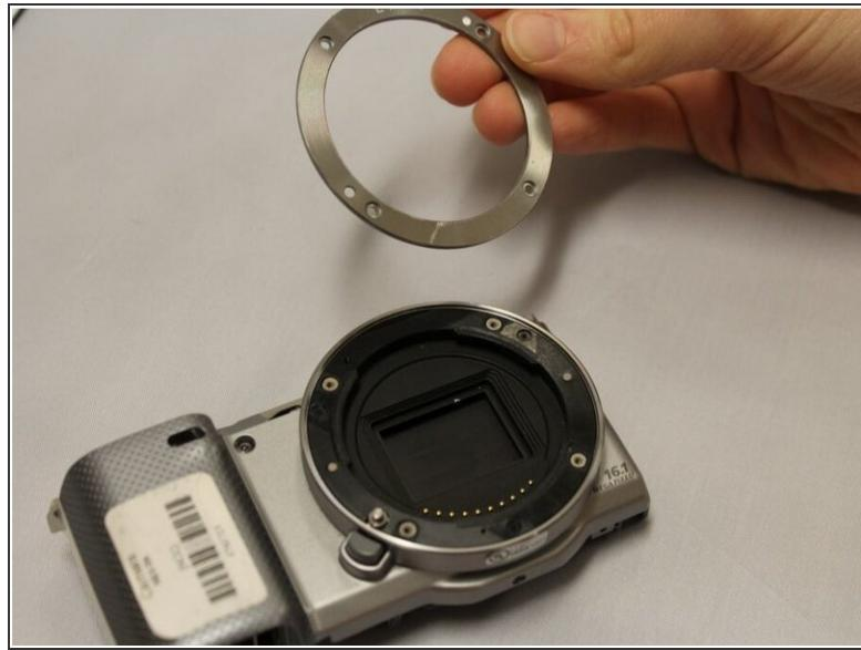
**⚠** While completing this guide, **do not** touch the **image sensor** (the center rectangle encircled by the lens mount).
