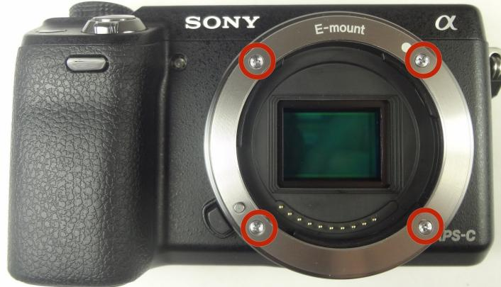
⚠ While dealing with this guide, **do not** touch the delicate **image sensor** (the center rectangle encircled by the lens mount).
