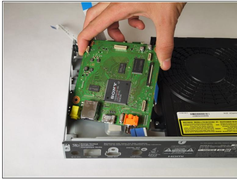
**⚠ Hold the motherboard exclusively by its sides as to not short it out or damage it irreparably.**
