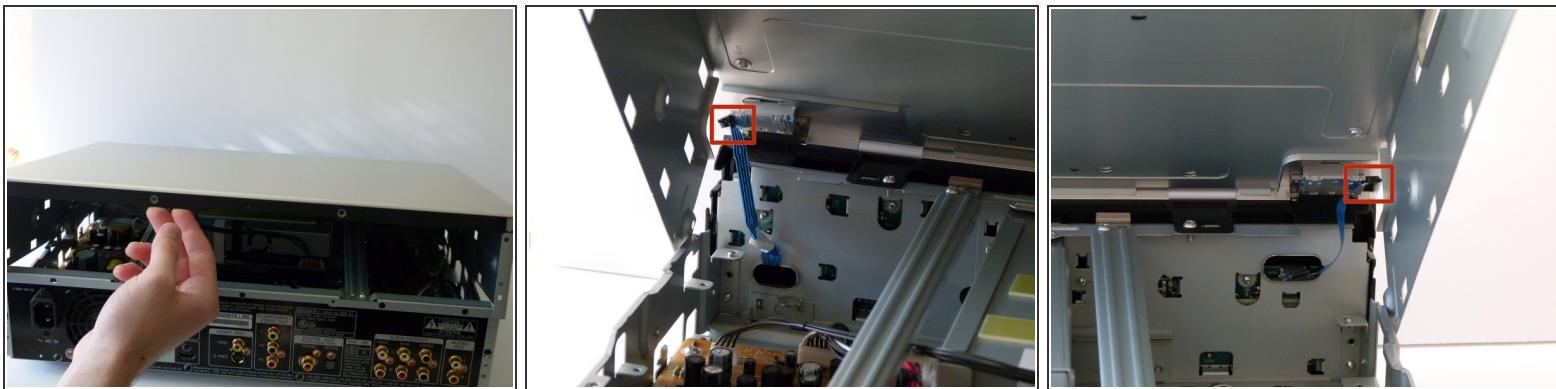
**⚠** Carefully lift up the top panel, because there are two blue ribbon cables that must be disconnected before removing the panel, and we do NOT want them to break.
