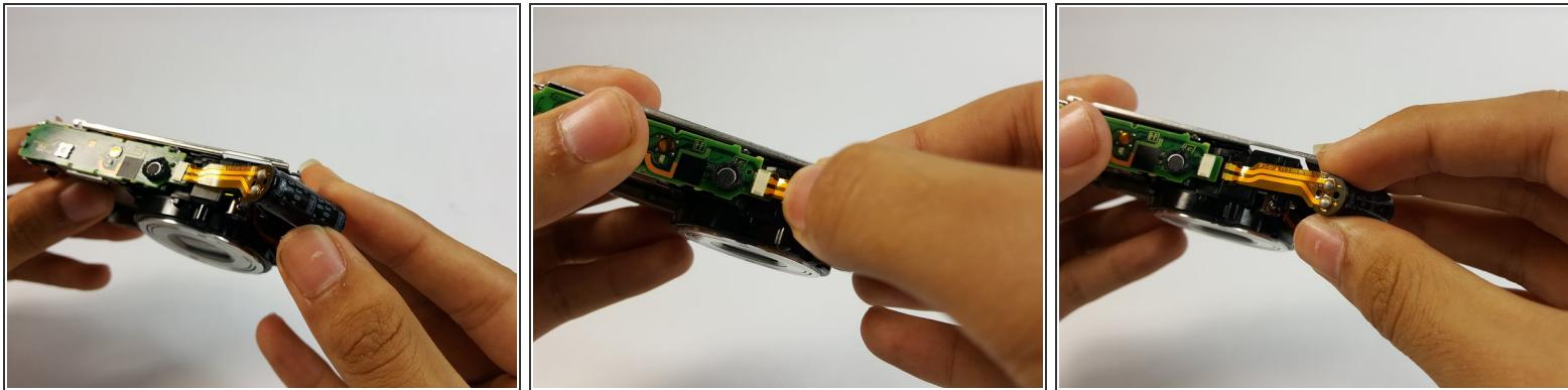
**⚠ Caution:** Be careful not to touch the capacitor wires as you work. If possible, use a [capacitor discharge probe](#) to safely rid the capacitors of dangerous charges.
