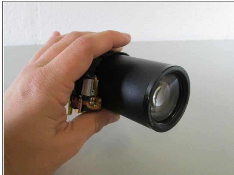
! The lens assembly contains exposed leads to capacitors. Be very careful to avoid contact or discharge capacitors before handling as touching the capacitors could lead to electric shock.
