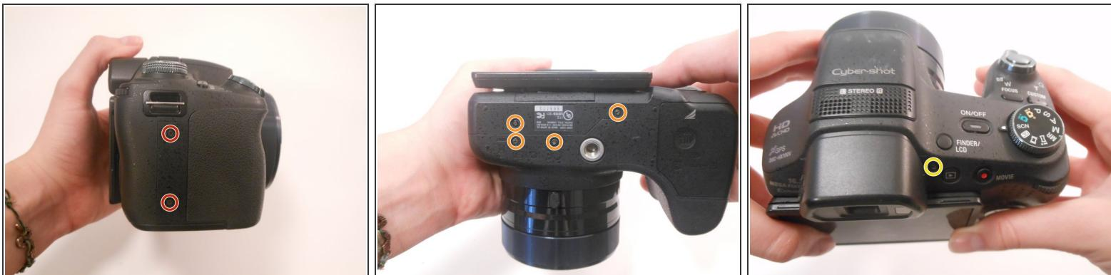
ⓘ Use the Phillips screwdriver size #00 to remove the 1.59mm #00 screws.
