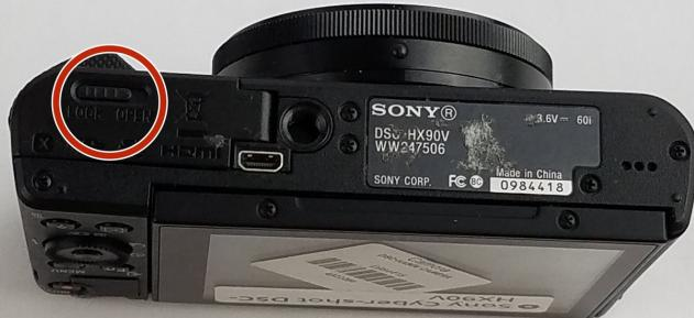
**i** Ensure the camera is turned off prior to the removal of the battery.
