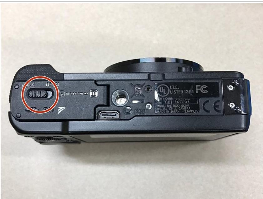
**i** Ensure the camera is powered off prior to removal of the battery. The LCD screen will have no information displayed if the camera is properly turned off.
