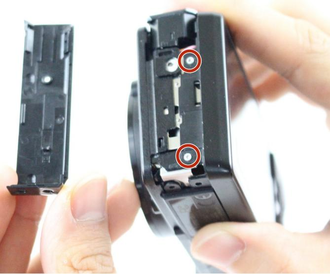
**⚠** The marked screws will loosen the rear case and the LCD screen may shift. The use of a soft work surface will prevent the LCD screen from breaking if it accidentally shifts during the removal process.
