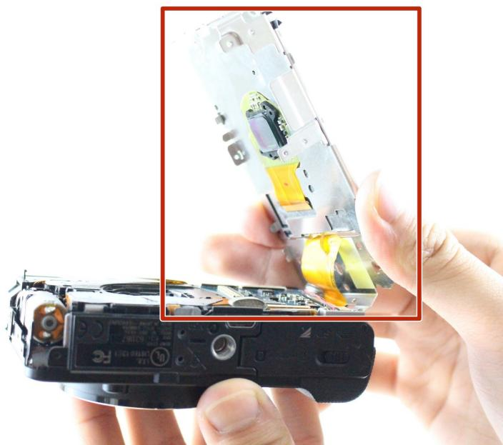
**⚠** LCD screen is very fragile. Handle with care. Do not use tools to remove the screen.
