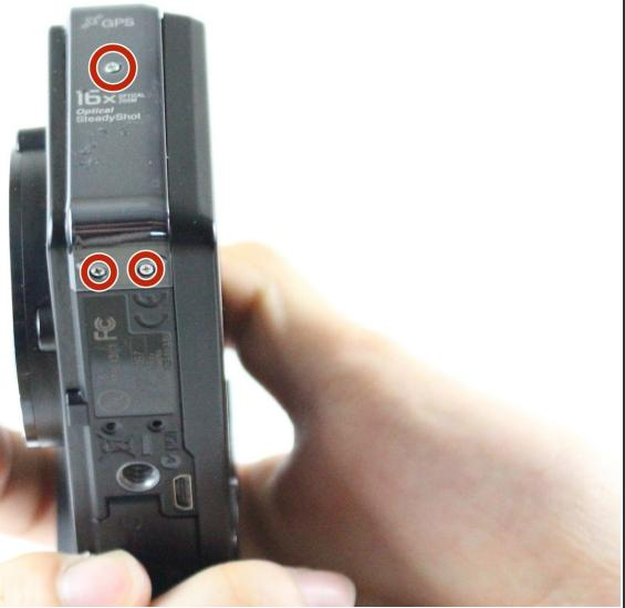
**i** The screws are very small and may become lost during removal. It is recommended to store the screws in a Ziplock bag or container until it is time to reassemble.
