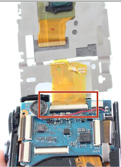
**⚠** Use caution when handling the data cable. Excessive force will permanently damage the cable.
