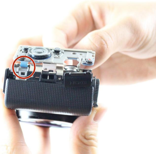
**⚠** Disconnect the control board data cable with care. Permanent damage may occur to the control board if tools are used to disconnect the data cable. Use your fingers only.
