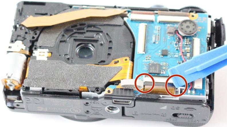
**⚠** Do not use excessive force to remove the lens data cable or permanent damage will occur to the cable.
