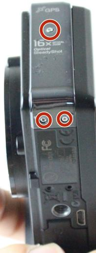
**i** The screws are very small and may become lost during removal. It is recommended to store the screws in a Ziplock bag or container until it is time to reassemble.
