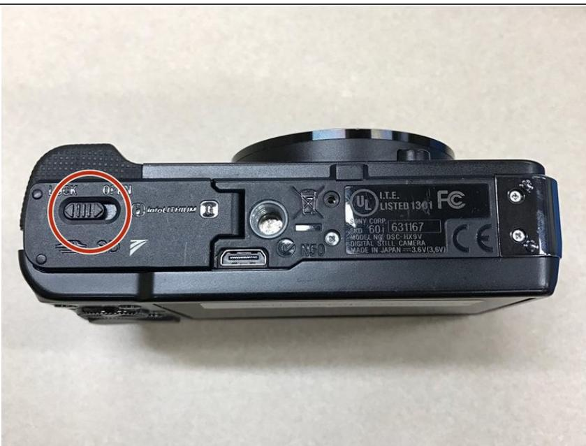
**i** Ensure the camera is powered off prior to removal of the battery. The LCD screen will have no information displayed if the camera is properly turned off.
