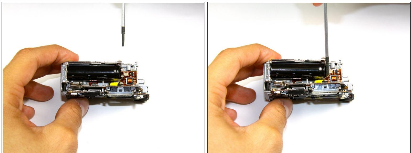
! Caution: the capacitor, a black cylinder near the top of the camera, might have a charge in it, which could be harmful to you or the camera. Neutralize it by touching both wires with a screwdriver at the same time.
