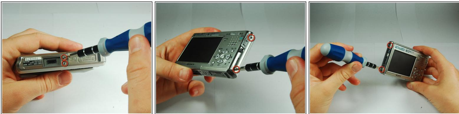
ⓘ There are two screws on the left and right sides of the camera, and two screws on the bottom.
