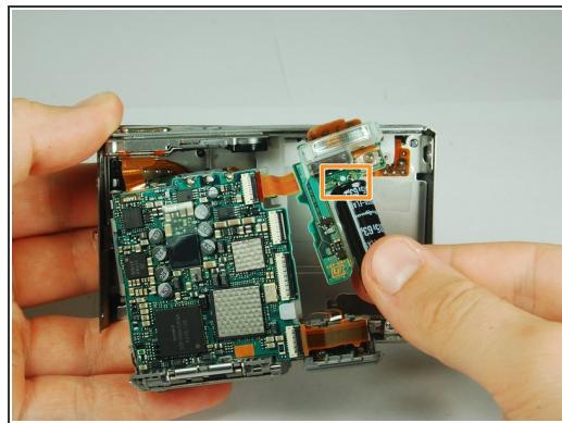
**⚠** This camera houses a very strong capacitor (the black cylinder). Avoid touching anything around the two wires coming out of the top. Doing so will risk serious electric shock.
