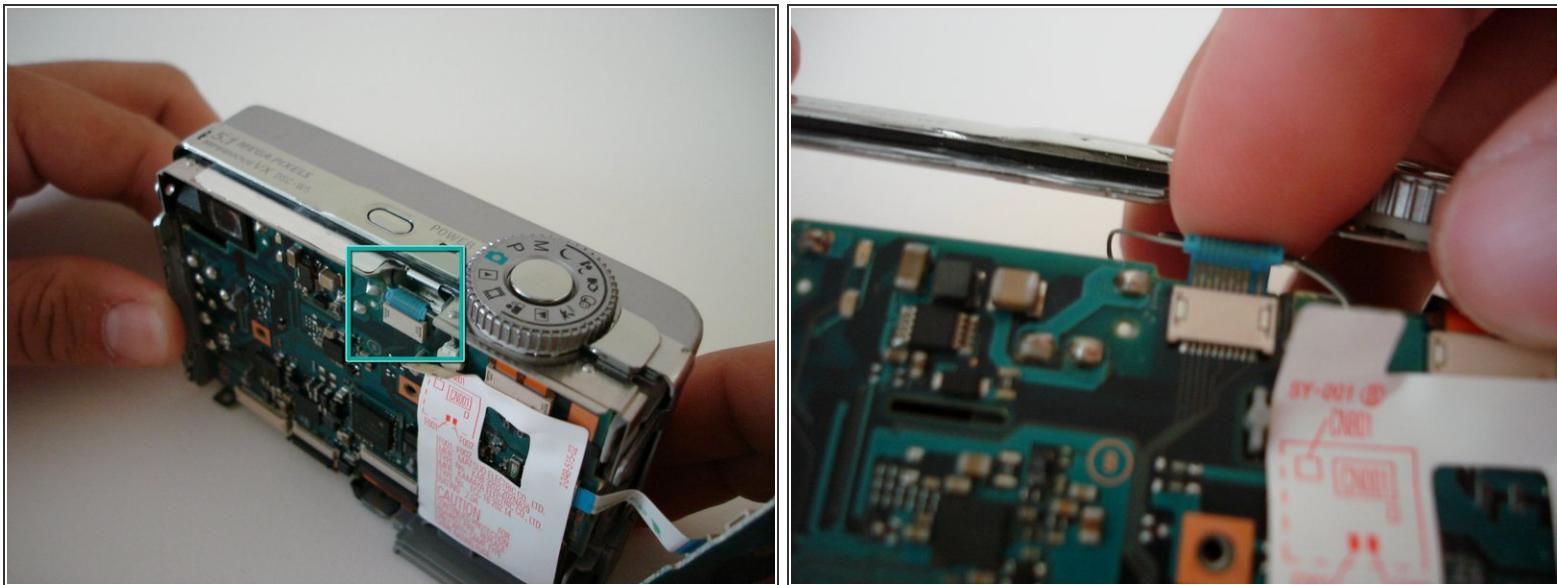
**⚠ Warning: Electric Shock** From this point on, hold the camera by the chrome edges ONLY. Capacitors store electric charge even if the batteries are removed.
