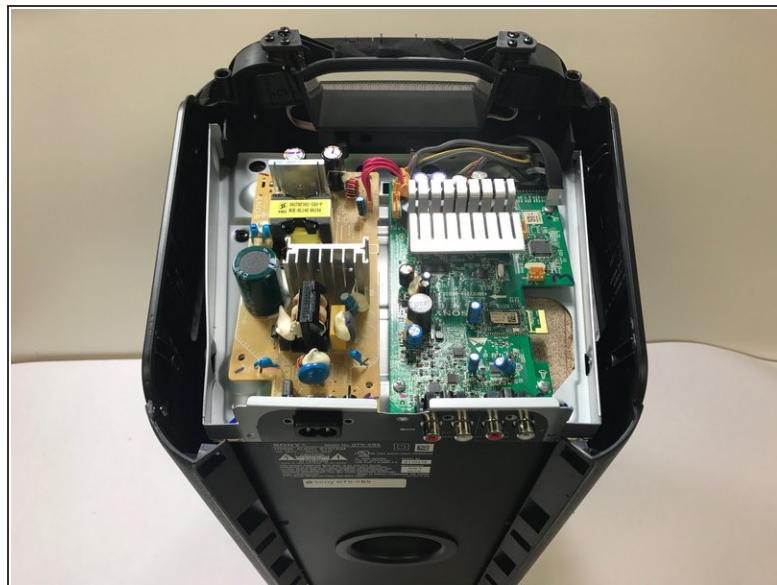
**⚠ Caution:** Be careful not to touch the capacitor wires as you work. If possible, use a [capacitor discharge probe](#) to safely rid the capacitors of dangerous charges.
