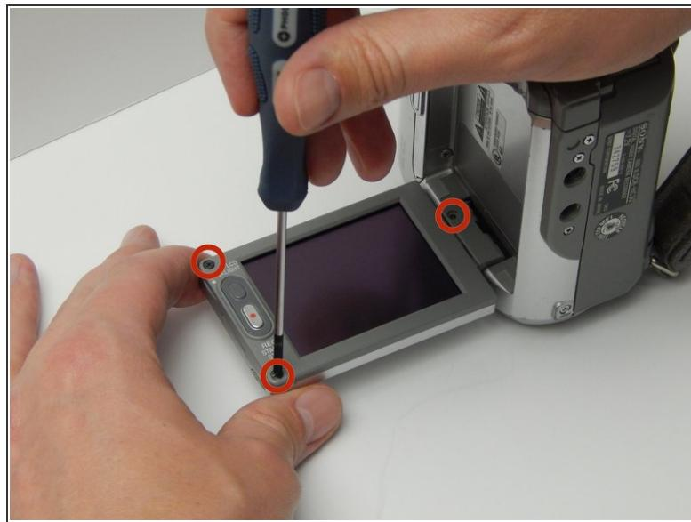
*(i)* To begin, the LCD screen must be removed.
